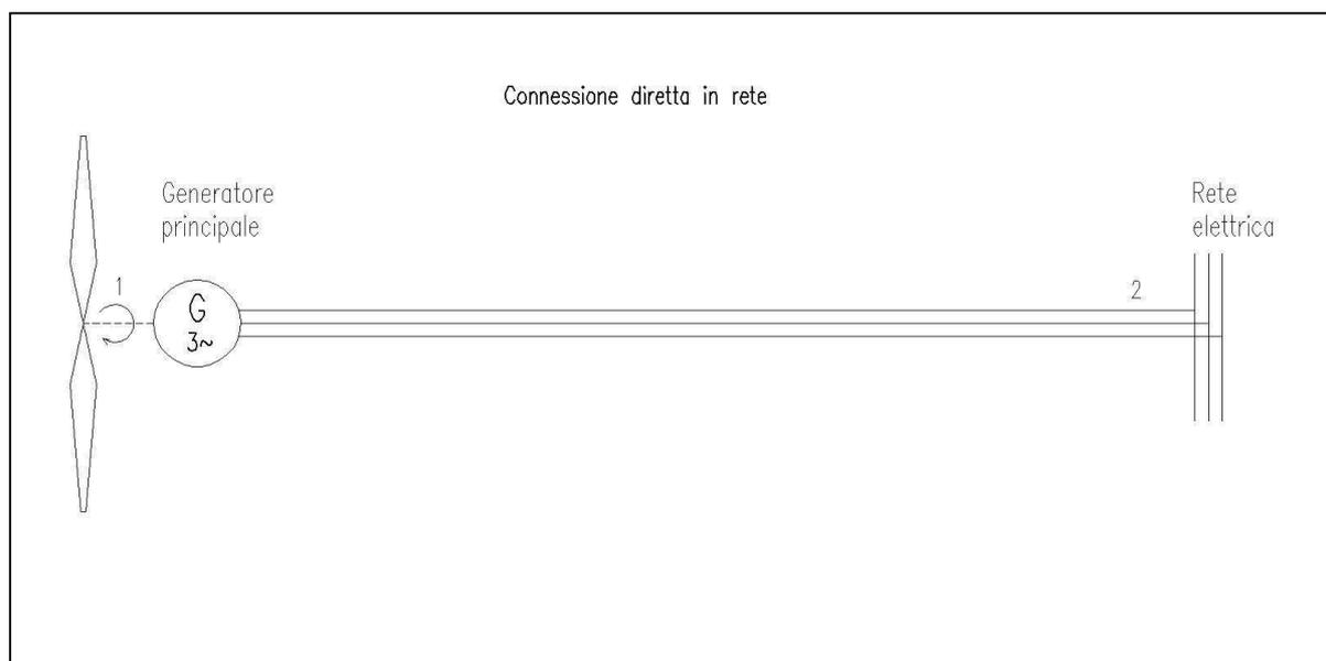
In order to operate, as the fixed frequency of the three phase voltage (point 2) is determined by the grid, the generator is required to rotate at a frequency that is almost identical to the grid (allowing for a small difference due to the necessary 'slip' that is typical of asynchronous electric machines). For this reason, the wind rotor will be forced to rotate at a steady speed practically equal to grid frequency speed.
