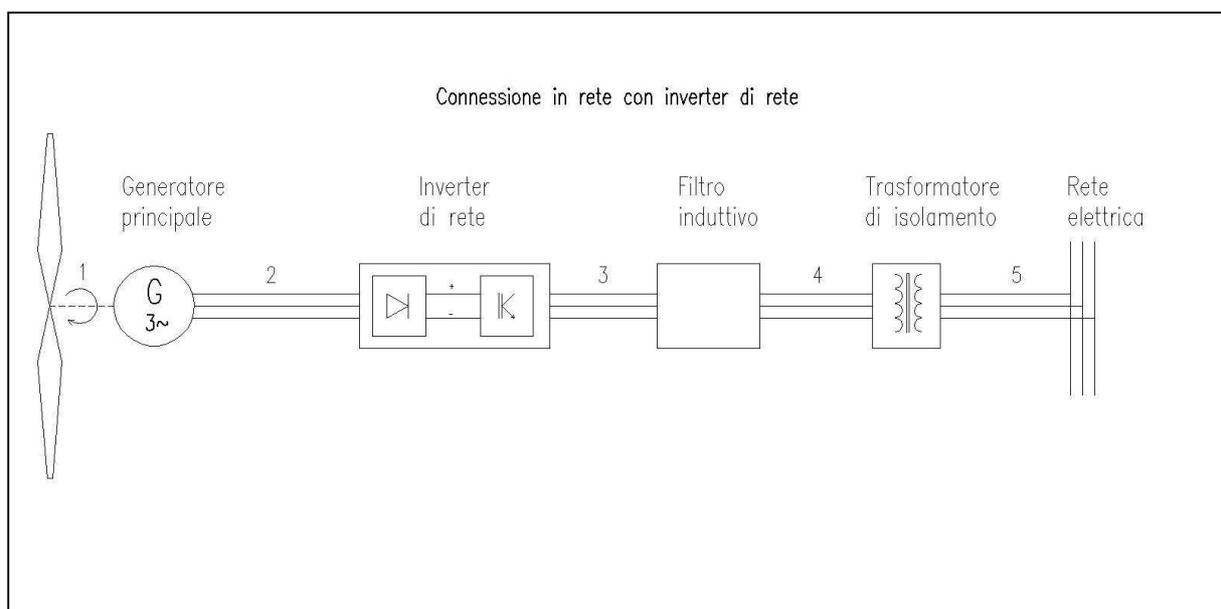
There will be a three-phase voltage variable both in voltage and frequency, for the number of rotations of the wind rotor (point 2).
