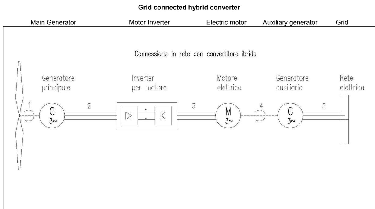
The drawing shows the grid connection principle of this type of conversion system: the wind causes the rotor to rotate, connected by the hub with appropriate transmission units (not shown) to the generator. In point 2 there will be a three-phase voltage, variable in value and frequency according to the number of rotations of the wind rotor.
