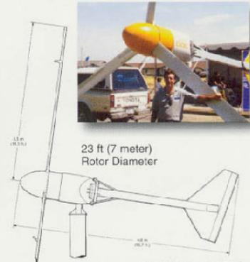
23 ft (7 meter) Rotor Diameter
